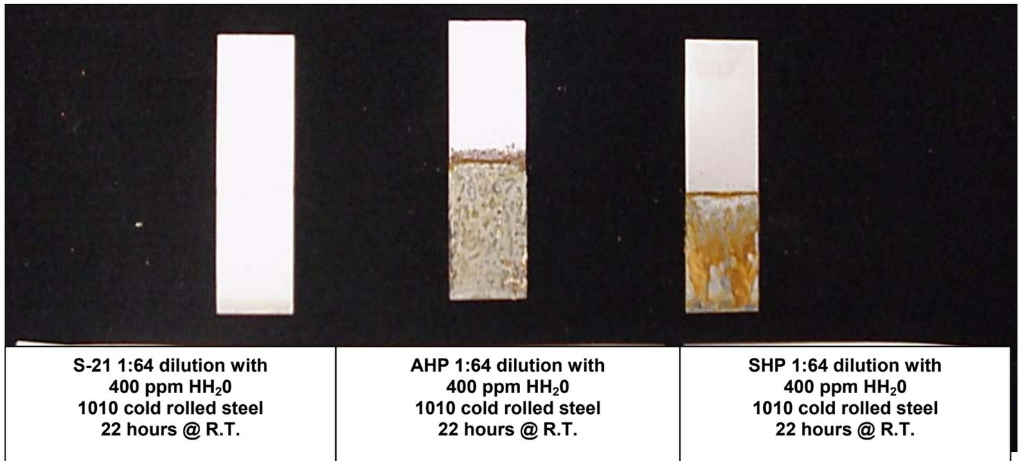
This shows how detrimental even slight splashing could be to metal surfaces when Hydrogen Peroxide formulations are used, even at use-dilution levels.
